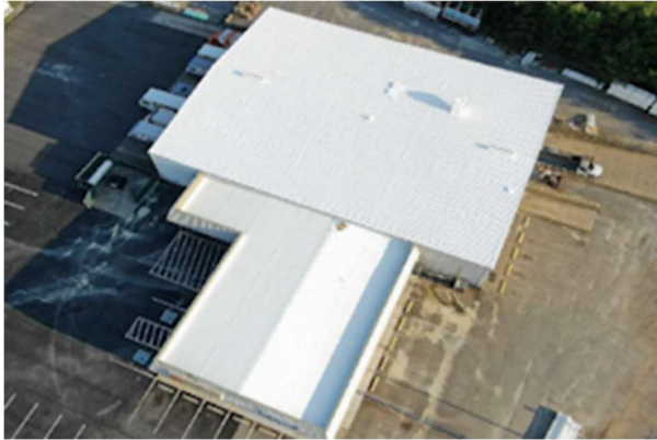
Roof are White for Maximum Reflectivity
